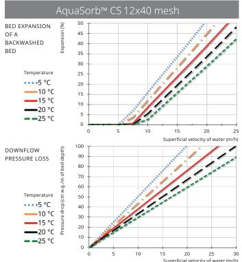
Bed expansion and pressure loss curves are provided for the most commonly used particle sizes. Charts are available for all particle sizes on request. Typical data only for indicative purposes.
